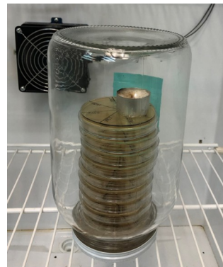
Mycoplasma grows best without oxygen. These jars with lit candles inside create an anaerobic environment where mycoplasma grows over 5-7 days.
